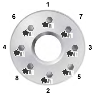
8-lug nut torque sequence
